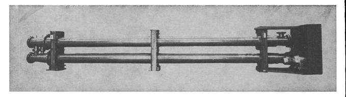
For use crystallizing: Tallow fatty acids, tall oil heads cuts and mid cuts, many neutral fats from vegetable, animal and marine sources, and cooling viscous materials.
